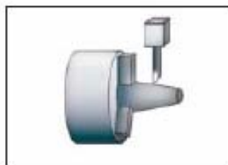
Accuracy of taper machining at constant surface speed is further improved due to faster internal arithmetic control and 10-nanometer interpolation control.
