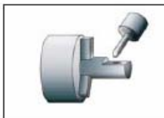
In milling on Y-Z plane using inclined Y-axis, travel in X-axis direction is reduced when the Y-axis is traveling.
